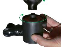
Purge air, then rotate cylinder counter-clockwise to remove
