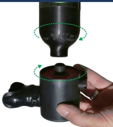
Purge air, then rotate cylinder counter-clockwise to remove
